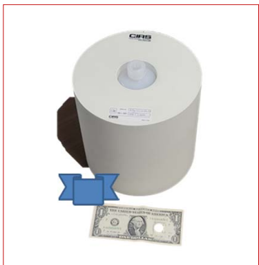
20 cm diameter certified tissue equivalent scatter/attenuation material phantom plus 250 ml sealable container for therapeutic radionuclide
